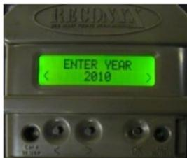
Press the << and >> buttons to scroll through settings for each step (year, month, day, hour, minute, temperature type and battery type); pressing the **OK** button after each step is entered correctly.
