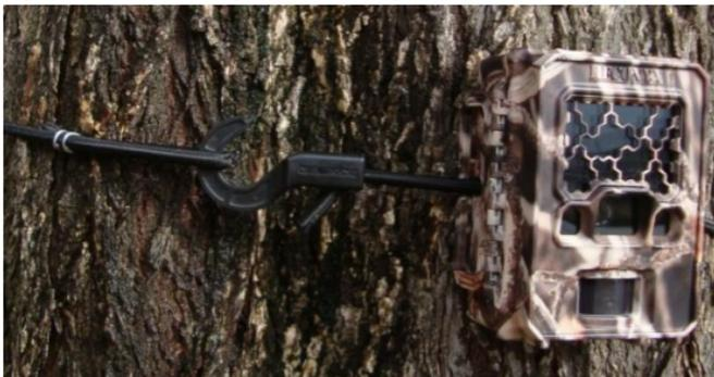
We recommend that you mount your camera about chest height and angle it slightly downward. This is optimal for detecting animals in the field of view of the camera as well as for accessing the camera's card, batteries, and controls.
