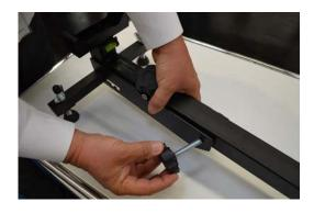
Insert the connector knob from the side opposite the welded nut so that it screws into the welded nut on the main frame. Be careful not to over tighten – the main frame should be able to move freely.
